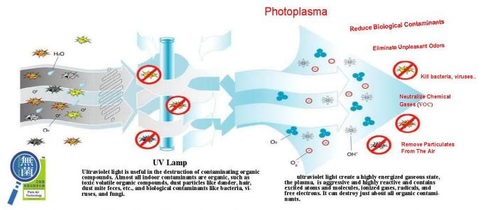
The key to the success of the unit's purifying methods is the creation of a cold gas plasma, is an excitation of gas by radio frequency energy — in our case, we excite gases by the energy from ultraviolet light waves. The plasma, or highly energized gaseous state, is aggressive and highly reactive and contains excited atoms and molecules, ionized gases, radicals, metastable particles, and free electrons. It can destroy a vast array of indoor contaminants
