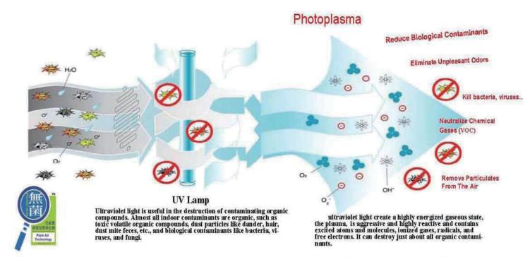
The key to the success of the unit's purifying methods is the creation of a cold gas plasma, is an excitation of gas by radio frequency energy — in our case, we excite gases by the energy from ultraviolet light waves. The plasma, or highly energized gaseous state, is aggressive and highly reactive and contains excited atoms and molecules, ionized gases, radicals, metastable particles, and free electrons. It can destroy a vast array of indoor contaminants
