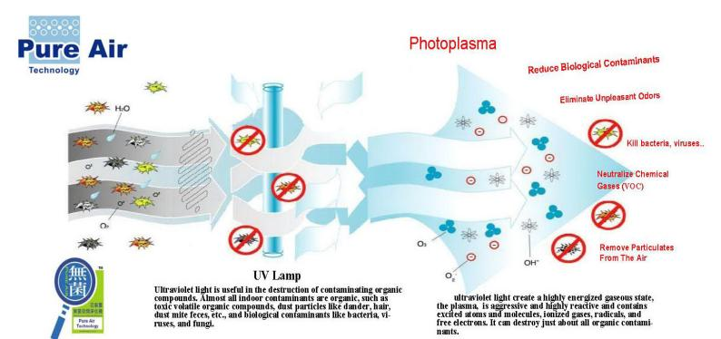
The key to the success of the unit's purifying methods is the creation of a cold gas plasma, is an excitation of gas by radio frequency energy — in our case, we excite gases by the energy from ultraviolet light waves. The plasma, or highly energized gaseous state, is aggressive and highly reactive and contains excited atoms and molecules, ionized gases, radicals, metastable particles, and free electrons. It can destroy a vast array of indoor contaminants
